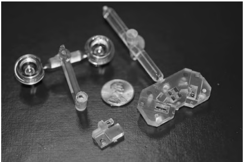
Figure 14.22 The replication of mini- and micro-optics by plastic injection molding
