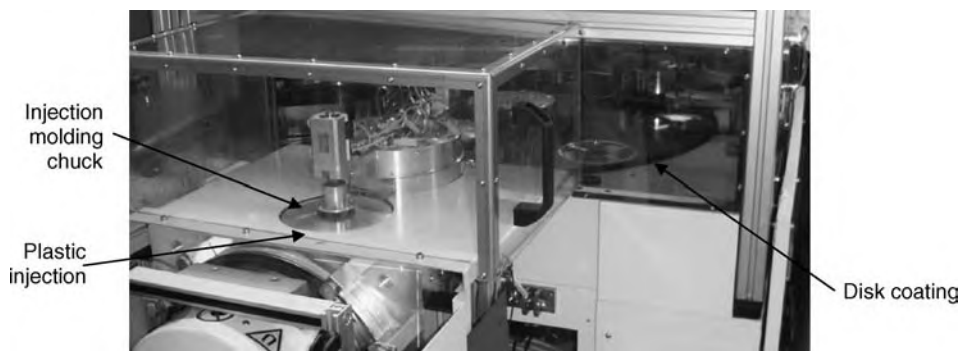
Figure 14.23 The CD injection molding replication process
