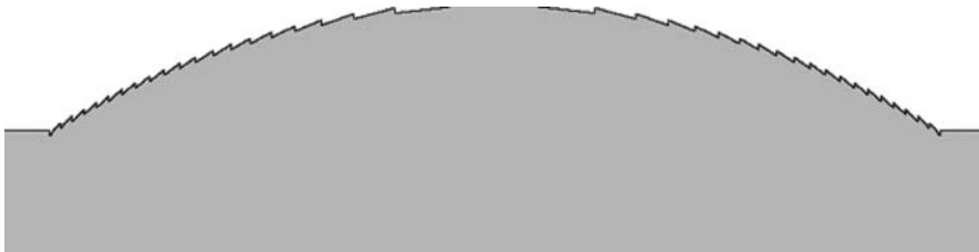
Figure 7.9 A hybrid achromatic singlet
